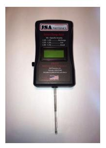
10,145,789) provides the user with a safe and convenient ability to directly measure the state-of-charge of open port, lead acid batteries commonly found in starting, lighting and ignition systems, stationary back up battery systems and motive power applications. Just insert the probe in the battery fluid, press the button and rapidly read the specific gravity of the cell.
